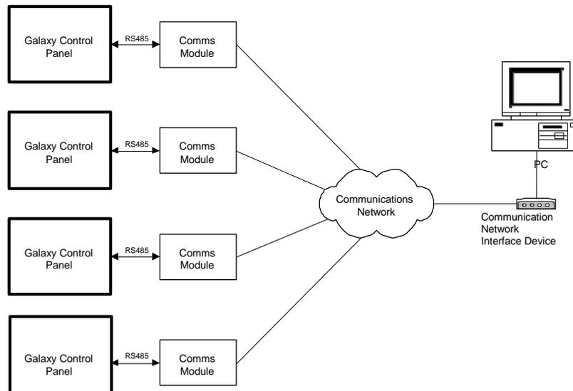
This type of configuration is designed for organisations requiring servicing and controlling multiple remote sites, enabling the information contained on each site to be copied, stored and overwritten using the PC. The stored information can also be modified using the off-line programming facility, enabling Galaxy sites to be programmed and stored on the PC in advance of commissioning the control panel.
