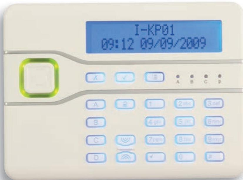
The i-kp01 is designed to work with i-on and Menvier control panels.
